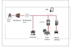
During the day, the solar panels installed on the roof of the carport use the photovoltaic effect to convert the solar energy directly into DC current, and convert the DC current into AC current through the inverter. The electricity generated can be used directly for the load. It can also be fed to the grid and stored by the energy storage battery for load at night.
